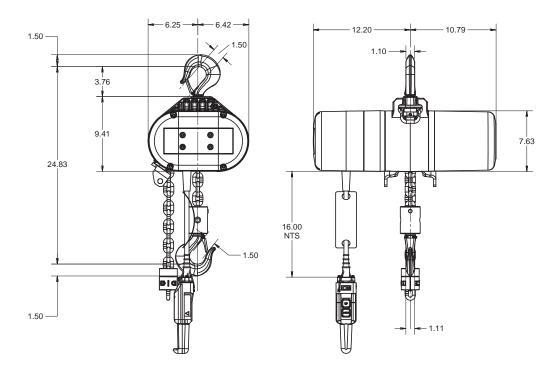
Dimensions (in inches) are RRS model CM Lodestar 2 Ton Single Reeved with Swivel Latch Type Hook Suspension.
